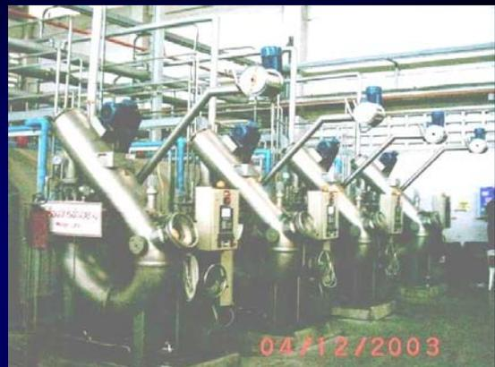
The new dyeing machine can dye at low and high temperatures. Steam passes through heat exchangers with condensate return and an accurate control system. The machine reduces chemical consumption per kilogram of product
